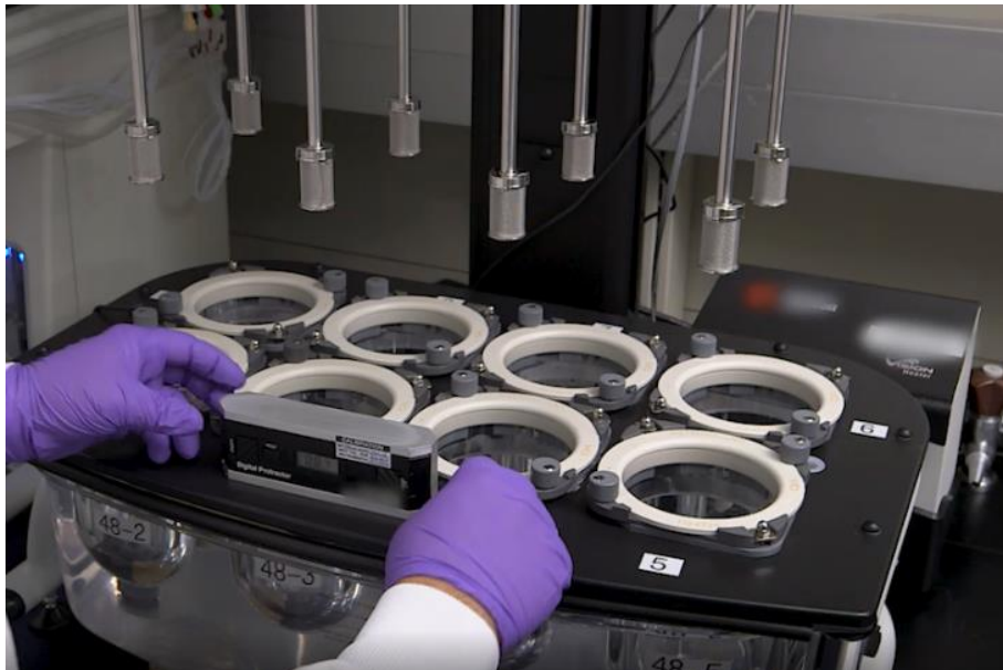
Figure 3. Measurement of vessel support plate levelness using electronic protractor.
