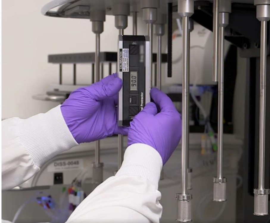
Figure 4. Measurement of shaft verticality using electronic protractor.
