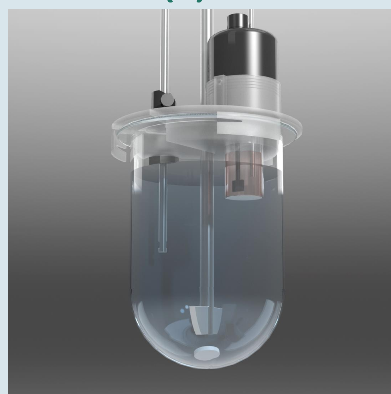
Figure 1. Schematic of Dissolution – Flux device used in this study
