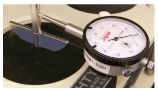
Figure 4. Dial test indicator (runout gauge) showing probe in contact with installed paddle shaft (Note that the measurement of basket wobble is similar with the probe tip in contact with the bottom basket rim). A different probe tip design may be used such as a large flat tip.
