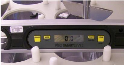
Figure 1. Electronic level giving  $0.0^{\circ}$  reading on the base plate of a test assembly.
