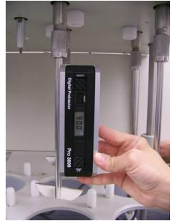
Figure 2. Measurement of the verticality of the stirring element using digital protractor.
